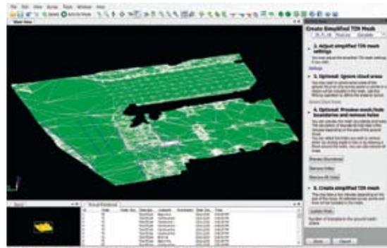
**Automatically removes buildings, cars, trees, noise, and generates a TIN surface.**
