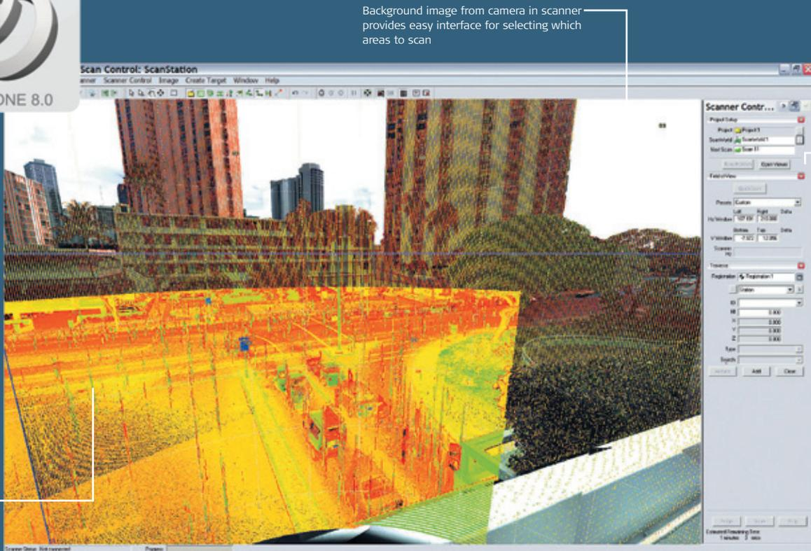
Background image from camera in scanner provides easy interface for selecting which areas to scan
